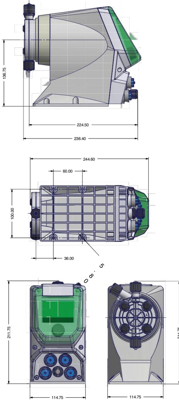
Fig. 3. Pump dimension - pump head mod. N
