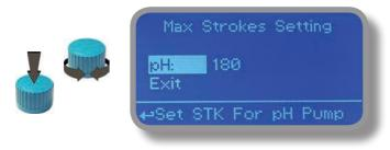
Note: Pump dosing capacity is based on 180 strokes per minutes
