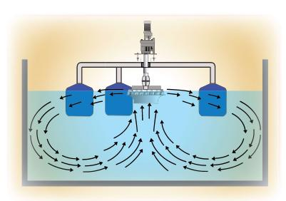
The deep pumping action of the Low Speed Surface Aerators / Francis Turbine Series generates effective I ocalized mixing to optimize many wastewater treatment processes. The Low Speed Surface Aerators / Francis Turbine Series is ideal for many industrial treatment process requiring fast and efficient oxygen transfer such as pulp and paper, food processing and others.
